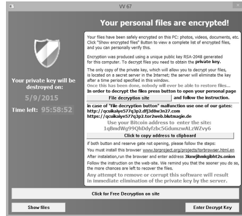
Fig. 1: The ransom demand from TeslaCrypt. The victim is instructed to access a Tor hidden service and pay the ransom with Bitcoin. Some variants allow the victim to recover a small number of files for free as a gesture of goodwill.
