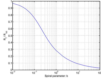
Figure 3: Ratio of the estimated dissemination radius between spiral and flooding
