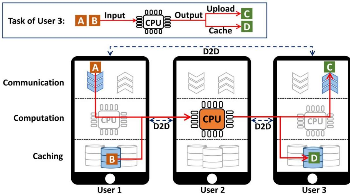
3C Resource Sharing based on D2D Cooperation (image from Ming Tang, Lin Gao, and Jianwei Huang, “Enabling Edge Cooperation in Tactile Internet via 3C Resource Sharing,” IEEE Journal on Selected Area in Communications, Special issue on Emerging Technologies in Tactile Internet and Backhaul/Fronthaul networks 2018)
