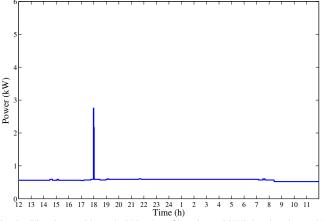
Fig. 4. The observed household load profile using a 5 kWh local rechargeable battery and an EV for load hiding.
