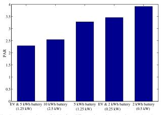
Fig. 7. Comparison of PAR for different batteries (maximum charging rate  $q_B^{\rm max}$ ) with and without the use of an EV for load hiding.
