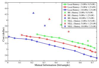
Fig. 5. Cost versus mutual information for different algorithms and batteries (maximum capacity  $C_B$  / maximum charging rate  $q_B^{max}$ ).
