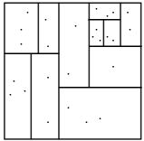
Figure 6: A kd-tree partitioning of a 2d-space
