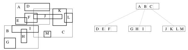
Figure 11: A set of rectangles represented by an R-tree
