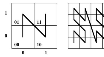
Figure 7: z-order enumeration of cells of a hierarchical partition
