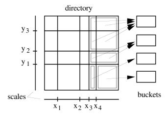
Figure 9: Structure of the grid file
