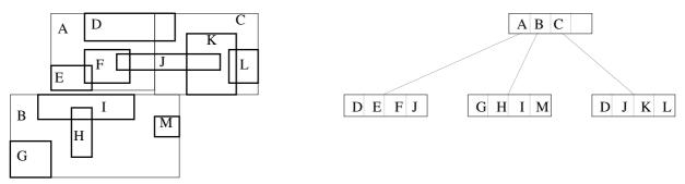
Figure 12: A set of rectangles represented by an R<sup>+</sup>-tree
