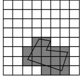
Figure 5: Bounding box and grid approximations of an SDT value
