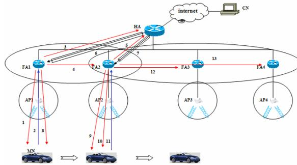
**Fig. 4.** Speed adaptive handoff procedure
