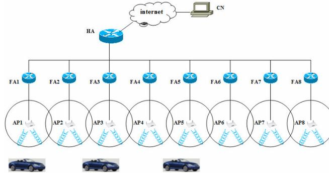
**Fig. 1.** Emulation scenario for MIP/ WLAN
