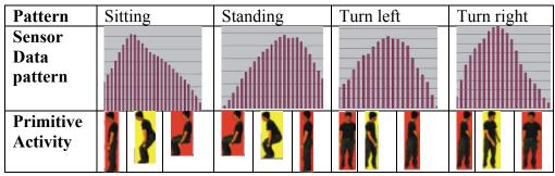
Figure 5. Extraction of motion patterns from sensor data [5]
