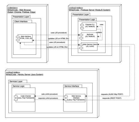
Fig. 5. Architecture: Deployment Diagram
