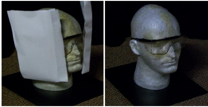
Figure 4. The glasses on the left limited FOV to 60 degrees, while the control glasses on the right did not reduce FOV.
