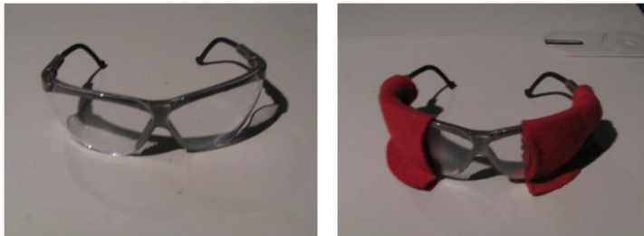
Figure 1. Unblocked goggles used in high FOV conditions (left); goggles with blinders used in low FOV conditions (right).
