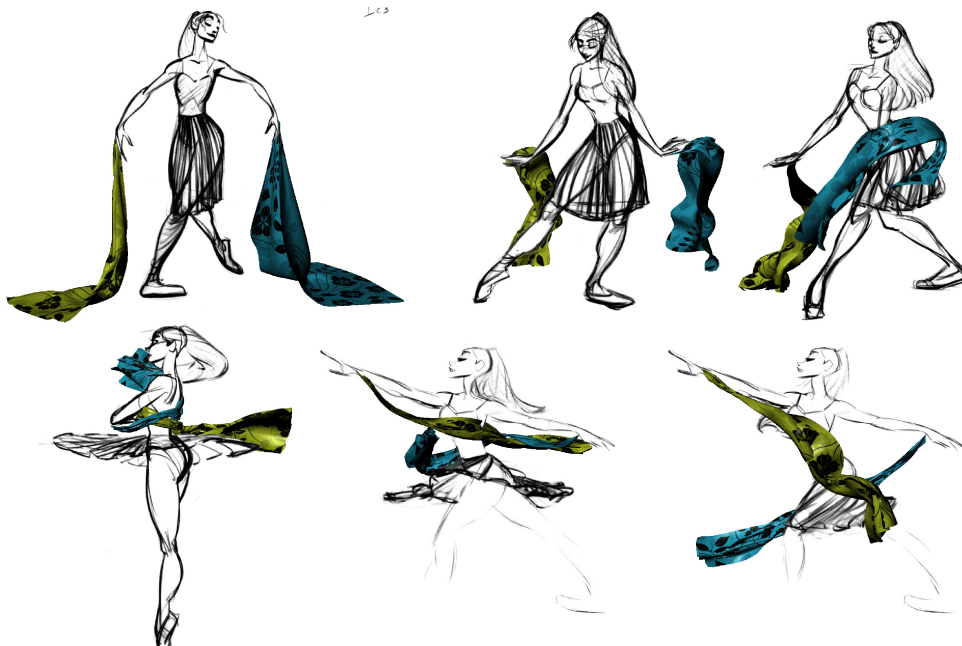
Figure 2.14: Ballet dancer: Scarves are simulated as 3D cloth. They are attached to the wrists of the dancer via single-point proxies for the wrist, and interact with the 3D cylinder proxy for the body of the hand-drawn ballerina, and thus, wrap around her waist.
