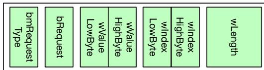
Fig. 8: Protocol fields used in the USB Setup packet in the Enumeration Procedure.
