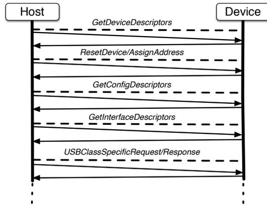
Fig. 7: USB Enumeration Procedure.
