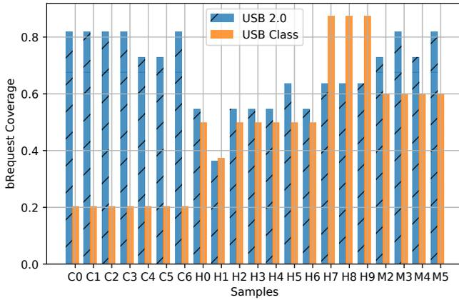
Fig. 15: bRequest value coverage comparing with different USB specifications for each firmware within the training set.
