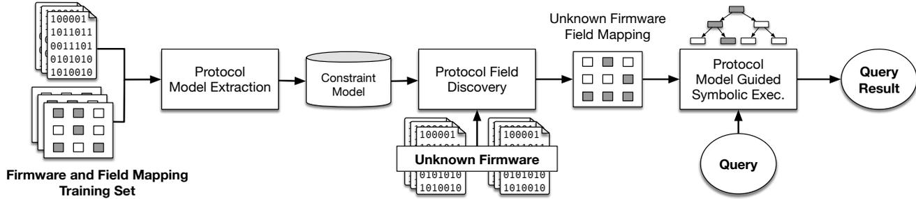
Fig. 1: ProXray: Protocol model extraction and its utilization in guided symbolic execution.
