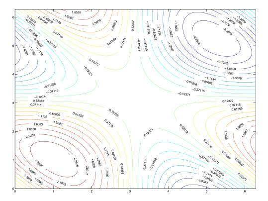
Figure 1: MATLAB plot of the level sets of the function  $f(x, y) = \sin x + \sin y + \sin(x + y)$ .
