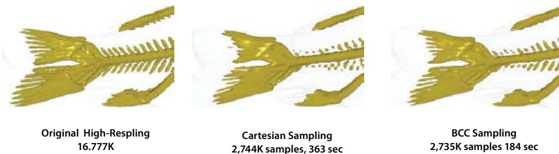
Figure 2: Visualizations of carp fish dataset. The optimal sampling improves the accuracy of imaging with the same number of samples. This is evident by the better reconstruction of the tail fins and ribs in the image rendered from the optimally sampled dataset. The optimally sampled image was rendered twice as fast as the Cartesian sampled dataset. These images are reconstructed by C2, fourth-order methods.
