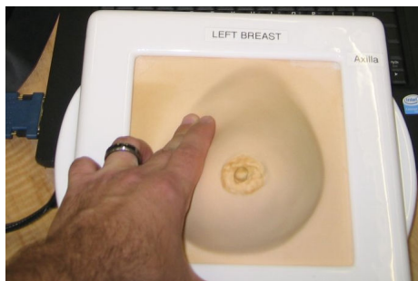
Figure 2. The physical breast simulator affords realistic soft-tissue haptic interaction and is used as a tangible interface to the MRH breast exam patient.
