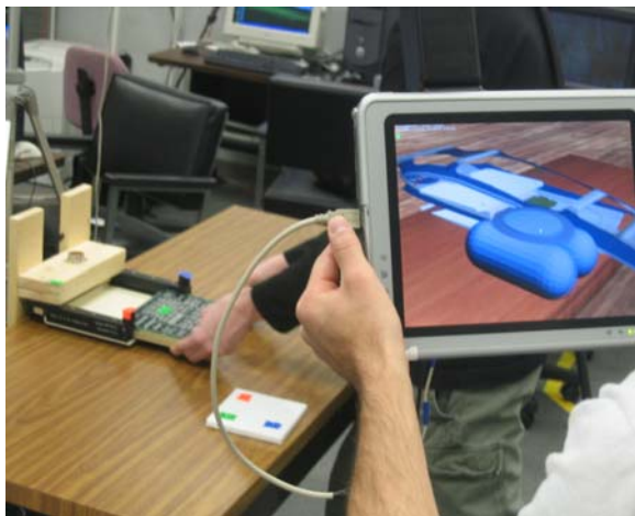
Figure 3. Secondary local users use a Magic Lens to view the virtual assembly procedure in the ME.
