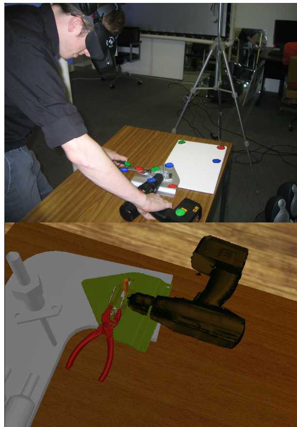
A user handles real objects and physical correlates ( top ), while visualizing articulated scanned models (pliers, drill), and a CAD model of a yet-to-be-built NASA payload component ( bottom ).
