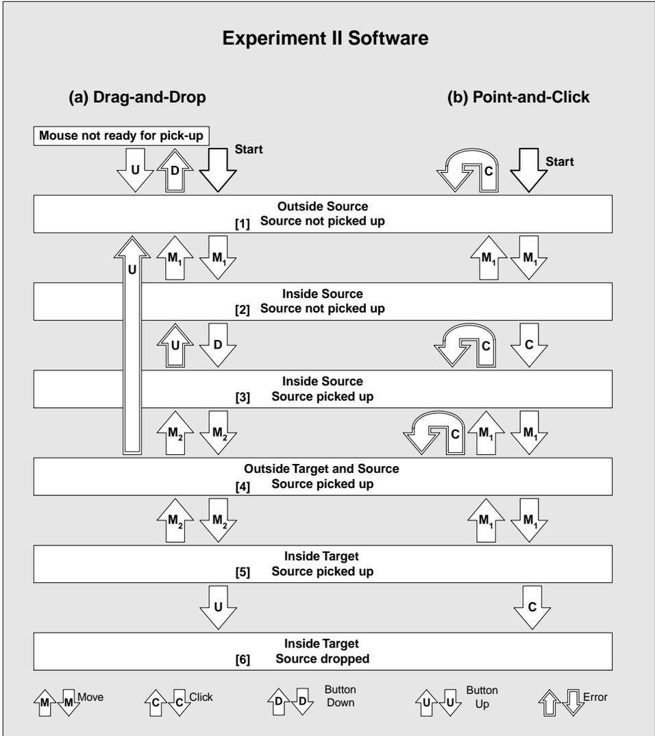
Fig. 5. State transition diagrams for (a) the drag-and-drop interaction style on the left and (b) the point-and-click interaction style on the right used in Experiment II.
