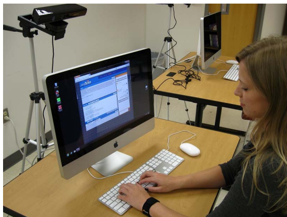
Figure 2. Student workstation with Kinect depth camera, skin conductance bracelet, and computer with webcam
