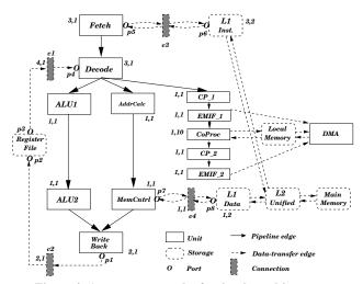
Figure 2. A structure graph of a simple architecture
