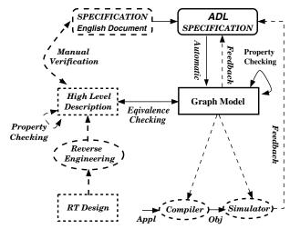
Figure 1. ADL-driven validation flow
