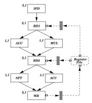
Figure 4. An example processor with false pipeline paths
