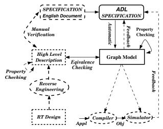
Figure 1. ADL-driven validation flow
