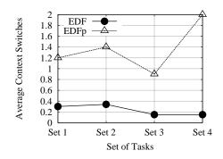
Fig. 12. Average number of context switches per task comparison between EDF and EDFp for various sets of tasks.
