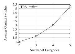
Fig. 11. Average number of context switches per task of task partitioning algorithm for various number of categories.
