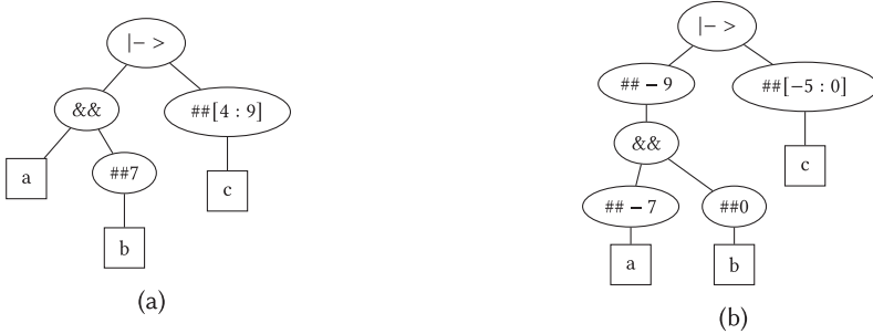
Fig. 5. (a) Simplified AST for \text{assert}(a \## 7 b \mid\text{-} > \##[4 : 9] c) . Logic operator, implication and delay are non-terminal nodes (oval), and others are terminals (rectangle). (b) Readjusted AST with timing. All delays are converted to local history values.
