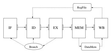
Fig. 19. The TLM Structure of an Alpha AXP Pipeline Processor
