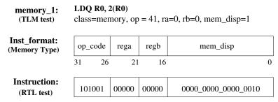
Fig. 22. The TLM to RTL instruction mapping of Alpha AXP Pipeline Processor
