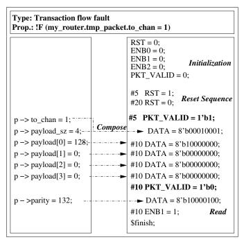
Fig. 18. TLM to RTL Test Transformation in the Router Example
