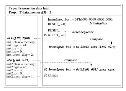
Fig. 23. TLM to RTL Test Transformation in the Alpha AXP Pipeline Processor
