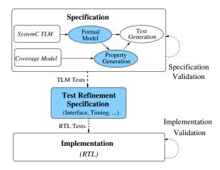
Fig. 1. Proposed RTL test generation methodology
