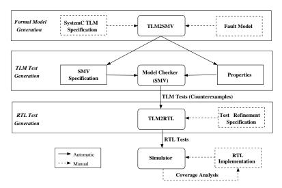
Fig. 13. The structure of our prototype tool
