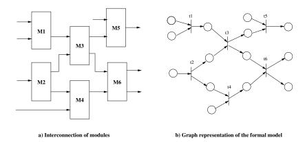
Fig. 2. Mapping from a SystemC structure to its corresponding formal model
