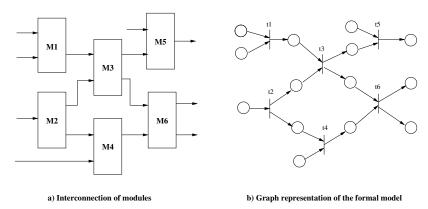
Fig. 2. Mapping from a SystemC structure to its corresponding formal model
