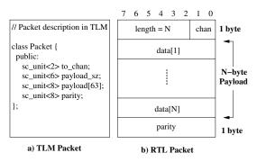
Fig. 15. The packet format of the router in TLM and RTL
