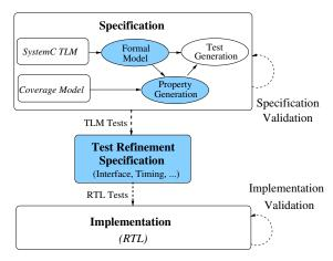
Fig. 1. Proposed RTL test generation methodology
