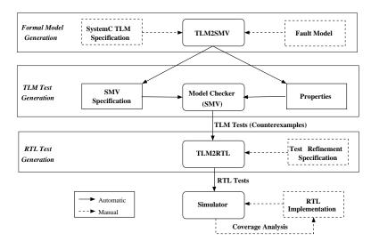
Fig. 13. The structure of our prototype tool
