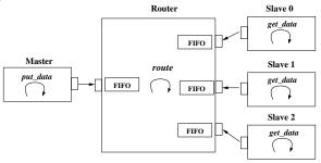
Fig. 14. The TLM structure of the router
