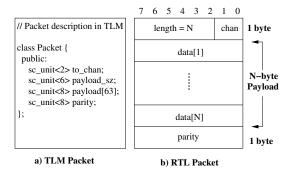
Fig. 15. The packet format of the router in TLM and RTL
