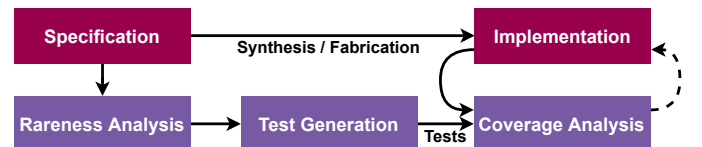
Fig. 2: Overview of test generation based Trojan detection
