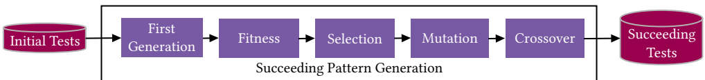
Fig. 10. Genetic algorithms based succeeding pattern generation for maximizing switching sensitivity for side-channel based Trojan detection in [80, 118]
