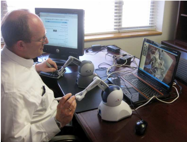
Figure 1: teaching module setup. The surgeon-author runs through the teaching module, setting the acceptable performance ranges. The monitor on the left, in the background, displays the web-based instructions, questionnaires, video, and the final feedback statistics. The other monitor, here a laptop, displays the 3D virtual scenario (run on the laptop). The interface consists of two Omni devices (robotic arms).
