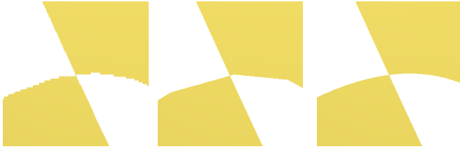
(a) insufficient scan resolution \mu_i (b) insufficient curve tessellation (c) correct resolution
