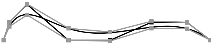
Fig. 2. A quintic spline and its envelope according to Corollary 1. The knots are at (0, 1, 3, 7) and the control points are (0, 1, 2, 0, 0, 1, 1, 0) . The first and last knot have multiplicity 6.
