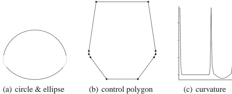
Figure 5:  $G^2$  spline **reproducing multiple conics**.
