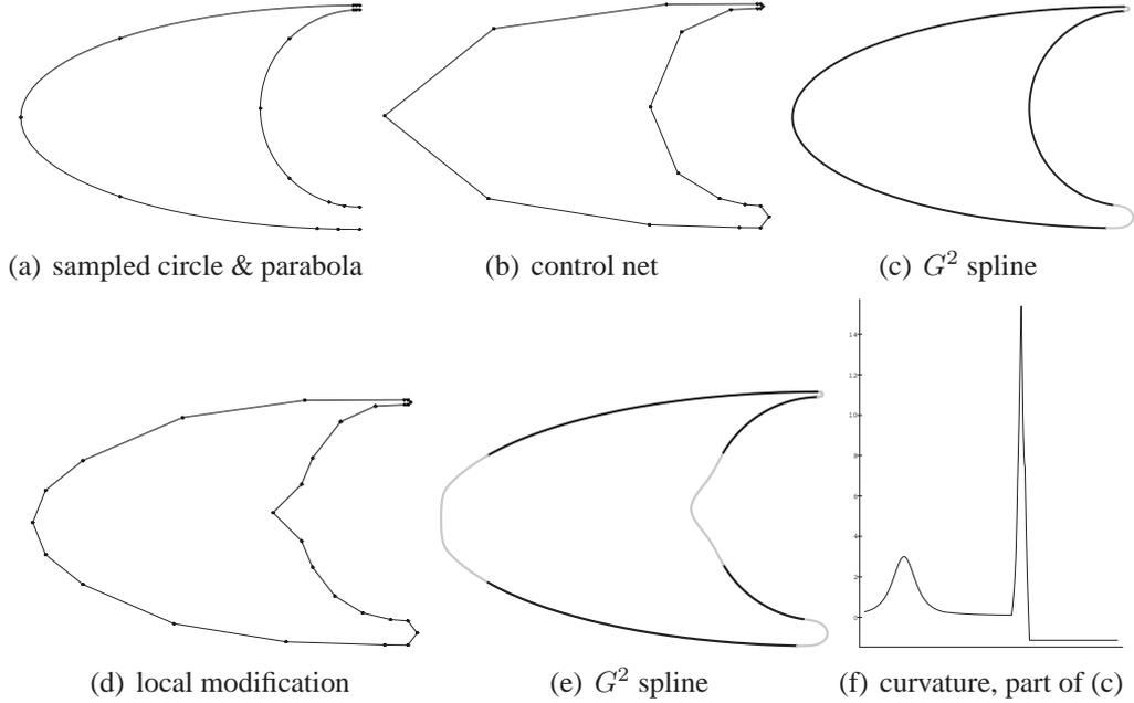
Figure 1: Exact reconstruction of conic pieces and localized blending.
