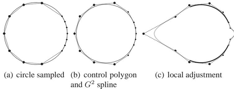
Figure 2: **Non-uniform spacing for local adjustment.** (a) A designer places points non-uniformly on the circle to initiate local adjustments. Small disks correspond to an opening angle of  $\pi/16$ , large ones to  $3\pi/16$ . (b) The derived control net and the exact circle generated by the  $G^2$  spline. (c) Local modification. Thick segments lie exactly on the circle.
