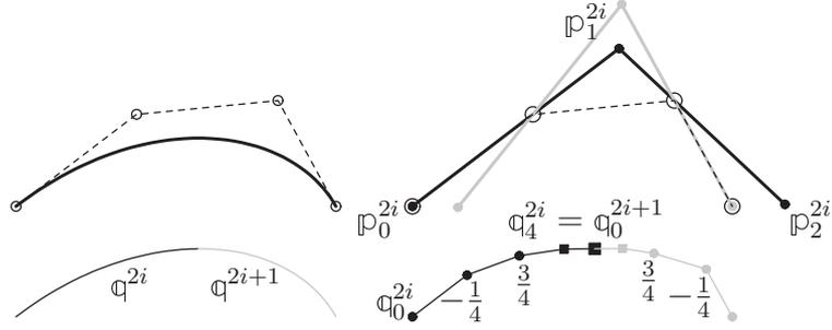
Figure 10: **Degree 4 splines derived from Hermite data.** (*top left*) A cubic  $G^2$  spline and (*top right*) its two 2-jets at the endpoints (cf. Fig. 9). (*bottom left*) The final of two quartic curve pieces and (*bottom right*) their control points.
