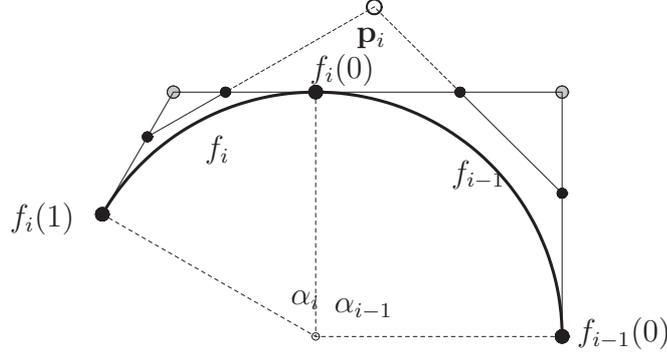
Figure 3: **Rational degree 3 representation of two adjacent arcs of a circle.** The middle coefficients of the quadratic pieces are shown as grey disks and the inner BB-coefficients  $\mathbf{b}_{i-1,1}$ ,  $\mathbf{b}_{i-1,2}$ ,  $\mathbf{b}_{i,1}$  and  $\mathbf{b}_{i,2}$  as black disks. The weights are  $w_{i0} = w_{i3} = 1$ ,  $w_{i1} = w_{i2} = \frac{1}{3} + \frac{2}{3} \cos \frac{\alpha_i}{2}$ .
