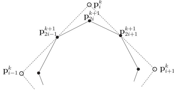
Figure 7: Refinement of a  $C^2$  spline control net.
