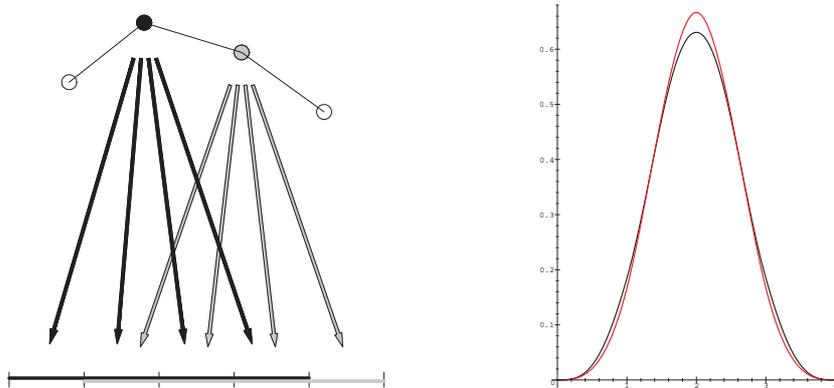
Figure 12: **Basis functions for rational cubic splines.** (*left*) Schema of influence. (*right*) Basis functions. The black curve is a uniform  $G^2$  cubic spline that reproduces a circle via arcs with an opening angle  $\pi/2$ ; the red curve is a uniform polynomial cubic  $C^2$  spline.
