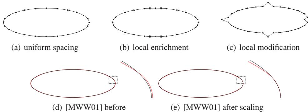
Figure 6: **Design modification** with the  $G^2$  rational cubic spline (a,b,c). (b) exactly reproduces the ellipse with non-uniform segments. (d) and (e) show two failed attempts at reproducing the ellipse with non-uniform segments using [MWW01] illustrating that it cannot be used for the localized modification.
