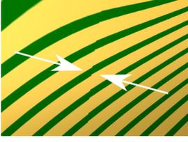
Figure 9: Highlight line mismatch visible under zoom (1/100 th of the edge length).
