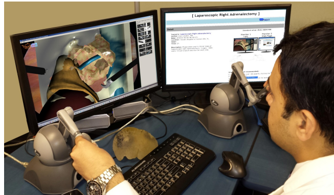
Figure 1. Computer simulated TIPS environment: left surgery simulation; right instructions, questionnaires, and video. Two low-cost ($2K/piece) six degrees-of-freedom haptic devices provide physical feedback.
