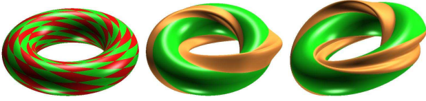
Fig. 9. A Villarceau parameterization of the torus offers different mesh layout and hence manipulation handles compared to Fig. 4 or 6.
