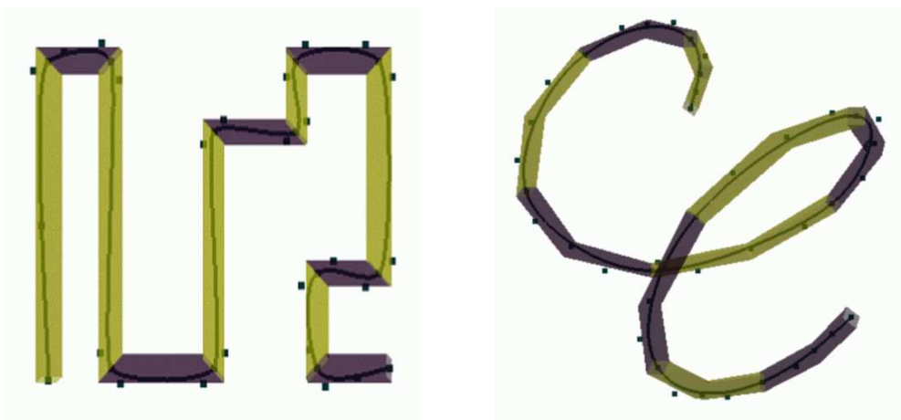
Fig. 13. ( left ) A 2D channel with 1 c-segment per c-piece. (c-pieces alternate in color). There is one piece of degree 3 per c-piece. ( right ) A 3D channel with two c-segments per c-piece. The spline curve is of degree 4.
