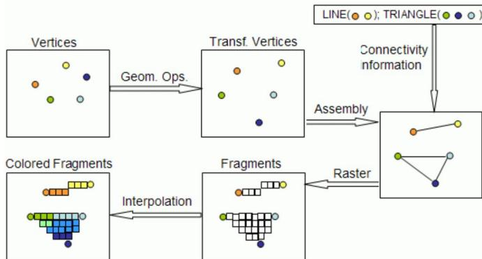
**Geometry processing:** 3D, floating point discrete
