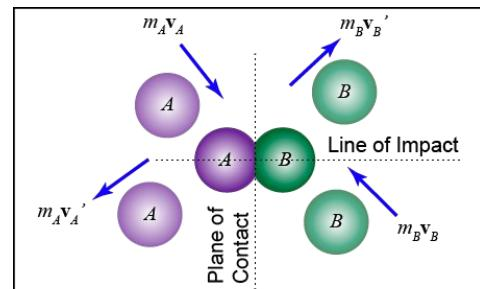
Figure 9.4-2: Line of impact and plane of contact
