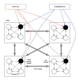
Fig. 1. Overview of the *lseb* simulator architecture. Threads communicate though IPC when on the same node, and over TCP sockets across nodes. The topology and command files control the simulation.
