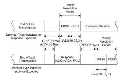
Figure 5. Interframe spacing in HomePlug 1.0
