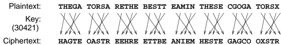
Figure 9: Example of a transposition cipher
