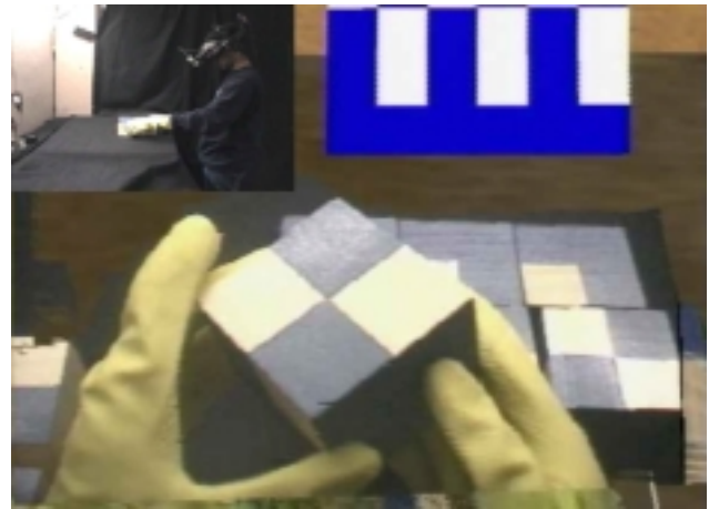
Figure 5 – Hybrid Environment (HE). Participant manipulated real objects while wearing dishwashing gloves to provide a generic avatar.
