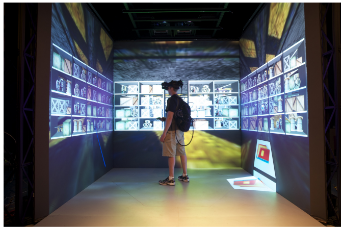
Fig. 2. This figure shows a user in the 270° CAVE while wearing the HMD setup. In the study, users only used one display at a time.
