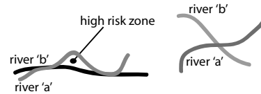
Figure 4: Two river scenarios, one with increased flood risk (left) and another with no increased flood risk (right).
