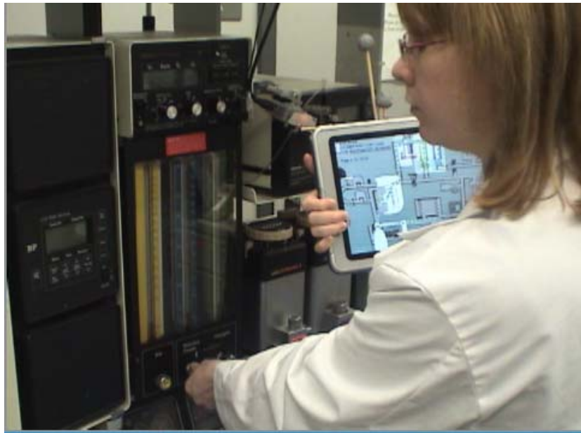
Figure 6.2: VAM-Context interaction: A user views how her interactions with the anesthesia machine affect the 2D VAM simulation.
