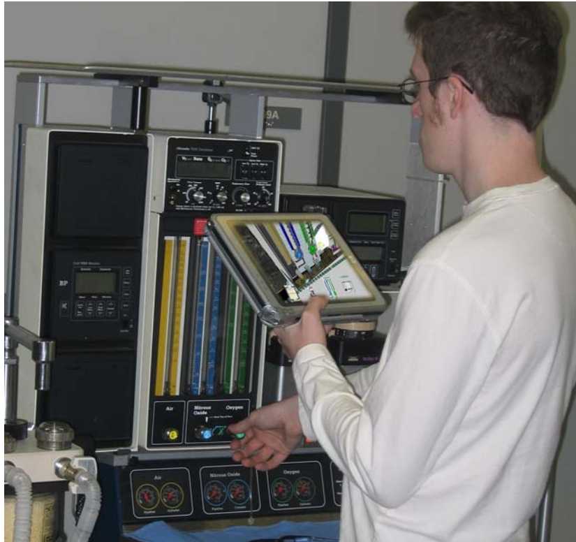
Figure 5.2. A user uses the real machine as an interface to the simulation. Thus, the simulation must be synchronized to the real machine.
