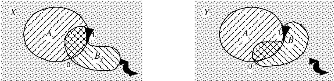
Figure 17: Two topologically distinct configurations that distinguish only by different inner/outer crossing types.
