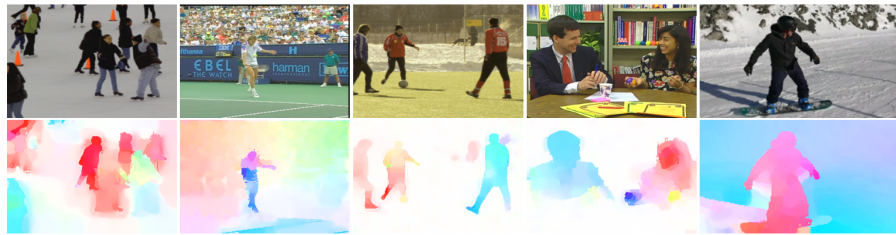
Figure 5: Examples of optical flow images. Top: RGB images. Bottom: corresponding motion magnitude estimates.
