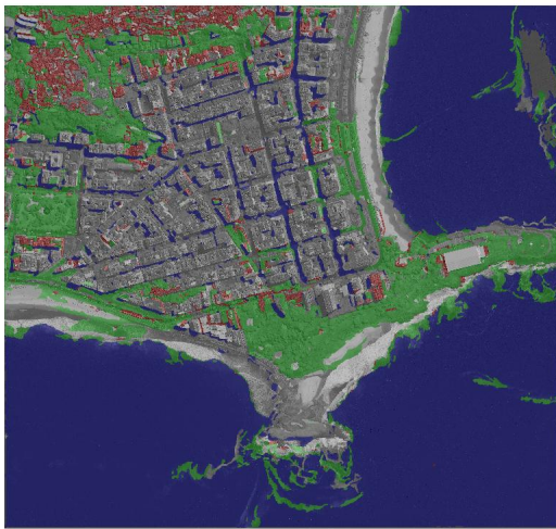
(c) Rudimentary classification obtained by SVM. The 5 categories are overlaid on the original image in different colors. Slums are shown by red, forests by green, urban by gray, sea with blue and sand shown as white.
