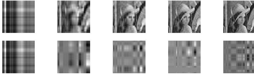
Fig. 2. Lenna reconstructions and components: Top row: Reconstructions using 1, 5, 10, 15 and 20 components. Bottom row: The SVD component images u_i v_i^T corresponding to the first five components.
