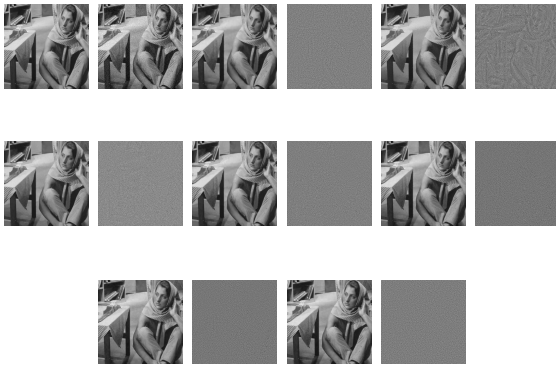
Fig. 5. Barbara image: left to right, top to bottom - clean image, noisy version with \sigma = 20 /PSNR = 22, output and residual for NL-SVD, NL-Means, BM3D1, BM3D2, HOSVD, HOSVD2, oracle. Zoom into pdf file for a detailed view. PSNR values in Table 1, image 12.
