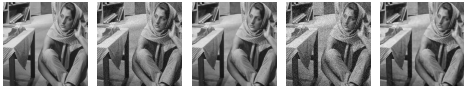
Fig. 3. Oracle filter with SVD: (left to right) clean Barbara image, noisy image with Gaussian noise of \sigma = 20 (PSNR = 22.11), filtered image with hard threshold 3\sigma in each patch (PSNR = 36.9), noisy image with Gaussian noise of \sigma = 40 (PSNR = 22.11), filtered image with hard threshold 3\sigma in each patch (PSNR = 31.34). Zoom into pdf file for a detailed view.
