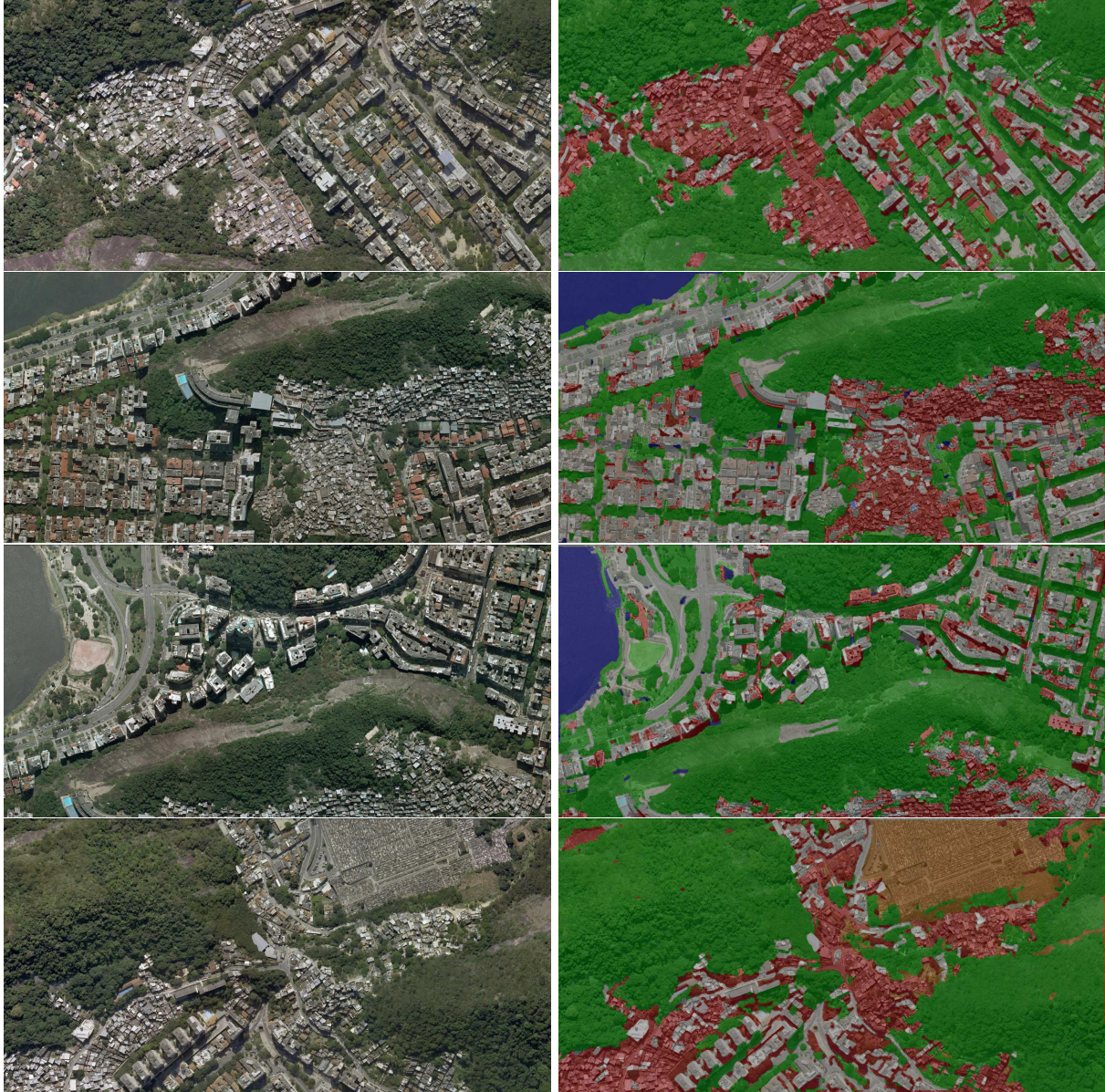
Figure 6: Results for 4 more images from Rio, Brazil. The left column shows the actual image and the right column corresponds to our GLSVM classification results. The colors red, gray, green, blue, and orange correspond to slum, urban, forest, sea, sand, and farm regions respectively.
