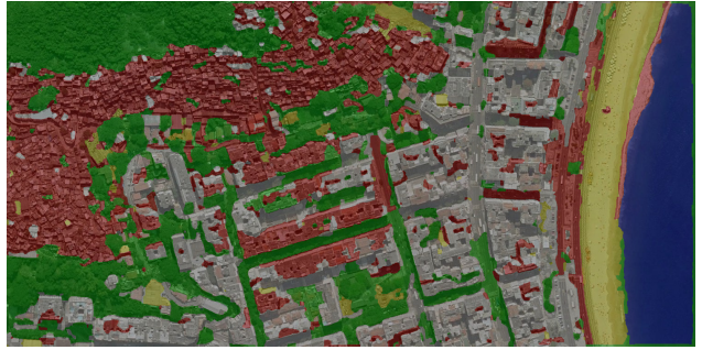
(b) Final result obtained after GLSVM. The output labels are smoothed during the model training.
