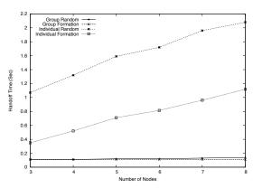
Fig. 4. The time required to perform successful handoffs for all nodes where the number of nodes per group varies. In these simulations, nodes were using DSDV to forward packets.
