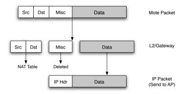
Fig. 3. An overview of the NAT-like packet processing in L2 nodes. Packets arrive at an L2 node on the interface corresponding to the mote networking protocol. The necessary data is removed and the process creates or checks a table entry corresponding to the source and destination addresses. The data is then placed in an IP packet and forwarded to its destination.
