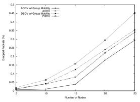
Fig. 6. The average packet loss for mobile nodes using the individual and group mobility mechanisms with the "random" movement model. For both AODV and DSDV, the group mobility method reduced dropped packets an average of 5 and 10%, respectively.
