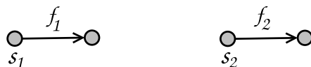
Figure 3-2. Two contending WLANs, where s_1 and s_2 are two access points. A TCP flow from a server on the Internet passes through an access point to a wireless node in each WLAN. Note that, only the wireless part of each flow (from an access point to a wireless client) is drawn in all figures throughout this chapter.
